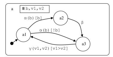
Figure 6. Variables, parameterised and transitional conditions
