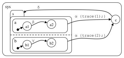
Figure 27. Race to a single target with traces [model t5472]
