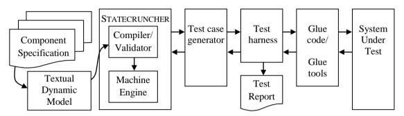
Figure 2. Compilation, Validation and Application to a Testing Tool Chain
